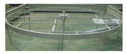
Test IFR at our factory. Note that the pontoons are not connected to the landing legs.
